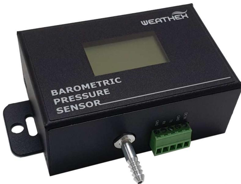
The **WxB-101L** utilizes internal silicon capacitive technology to measure atmospheric pressure. This method ensures long-term stability and high precision in pressure measurements. The measured pressure data is displayed on the LCD window through an RS-232 interface and protocol.
